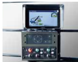
The high-visibility multifunctional moment limiter can be set easily with an interactive interface
