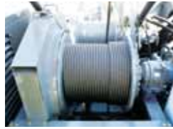
Drum with integrated reduction gear (winch with free fall function)
