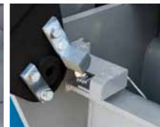
Secondary boom hoist limiting device that cannot be released by the operator
