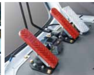
Winch with free fall function (brake pedals)
