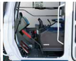
A gate lock lever keeps the crane safe against accidental operations
