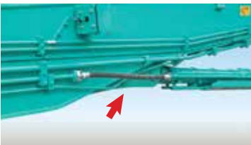
Hoses routed to protect from damages
