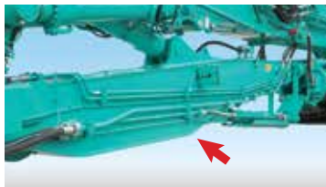
Electric wiring with optimized routing and full cover for preventing damage
