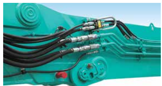
Piping connection: Hydraulic multi-coupler system on the side of the boom.
