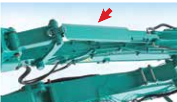
Guided reinforced bucket cylinder guard with box-type structure
