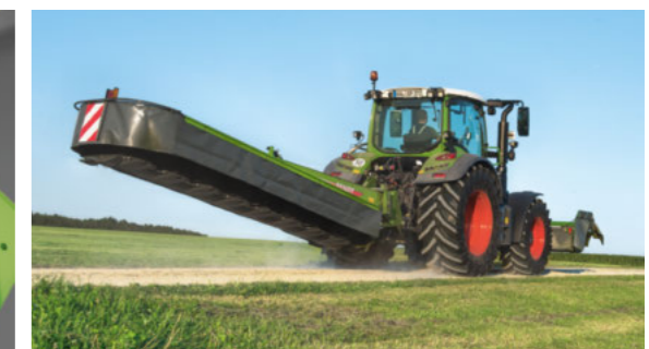
The mower swings through 90° to the rear from the cab in the transport position.
