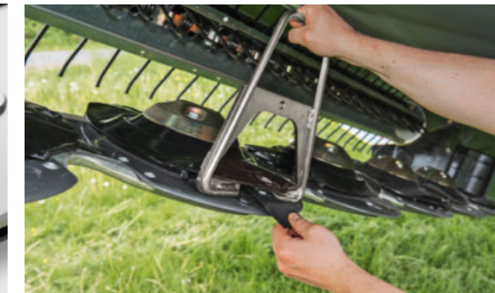
The convenient ComfortChange quick-release knife system makes maintenance child's play.
