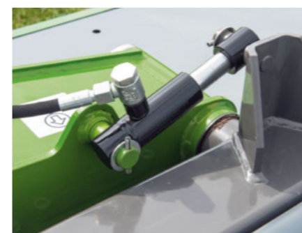
The compensation cylinder stabilises the mower unit on headlands and on the roads.
