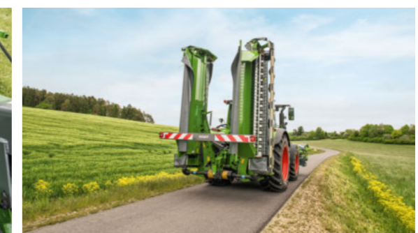
When folded, the mower combination remains below 4 m in height, and can be easily driven thanks to the low centre of gravity.
