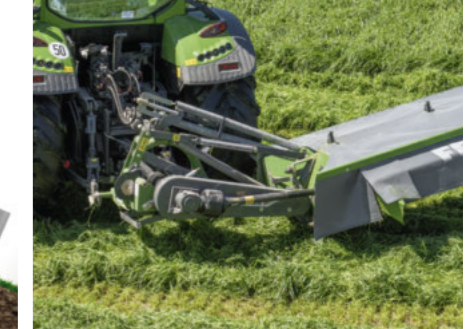
The spring-mounting ensures low ground pressure and protects the sward.
