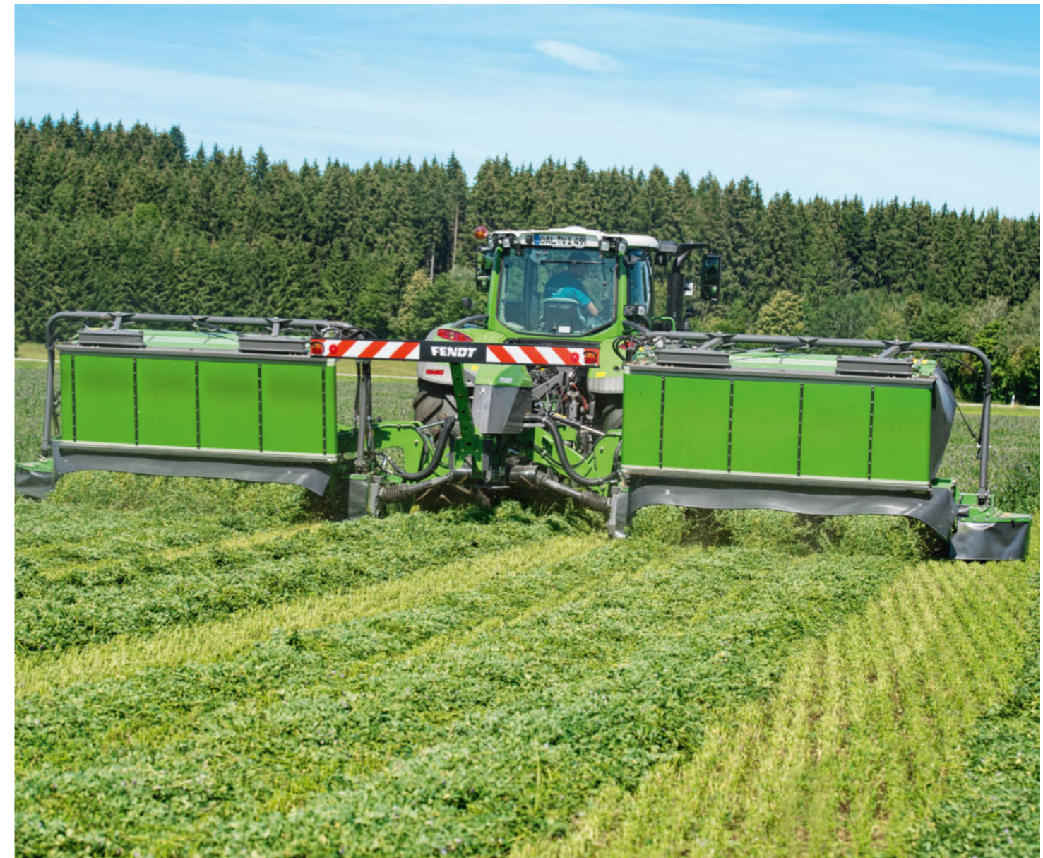
The belts can be folded up and the crop discharged across the full width at the touch of a button.
