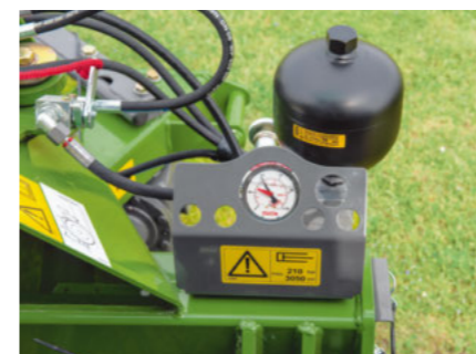
The hydropneumatic TurboLift cutterbed relief enables a single, floating cut.
