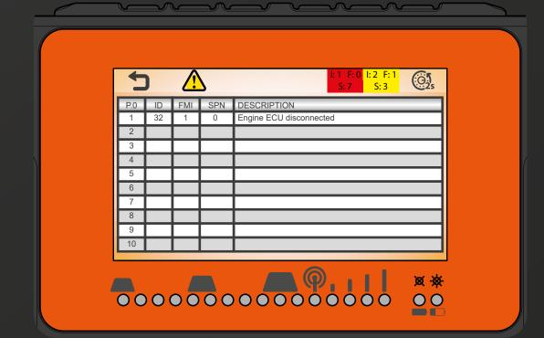
In case of wrong use or malfunctioning, a textual description of the error is reported directly on the display
