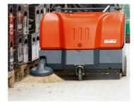
Cleaning close to edges; widely overlapping side broom provides easy working in curves.
