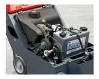
Maintenance-free batterypowered drive system: The on-board charger allows charging at any power outlet.
