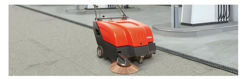
Optimised for small to medium-sized areas: The Sweepmaster 800 provides superior cleaning results with a sweeping performance of up to 4,350  $\rm m^2/h$ . This machine works by applying the clever overhead throwing principle which ensures maximum filling of the dirt hopper to provide both uninterrupted working and excellent sweeping results. The robust, heavyduty steel frame design makes this Sweepmaster a genuine professional – for impeccably clean floors at all times.
