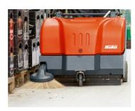
Cleaning close to edges; widely overlapping side broom provides easy working in curves.
