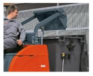
Comfortable high dump: At the push of a button, the dirt hopper can be emptied directly into any customary waste container (option).
