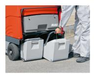
Take-it-Easy: The two dirt hoppers can be removed separately and emptied with ease. The hopper lifting system is particularly easy to operate and allows checking the filling level or throwing coarse pieces of debris into the hoppers at any time.
