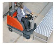
Manoeuvrability: Small turning circle even in particularly confined areas – thanks to the 90-degree steering angle.
