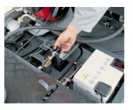
Adjusting the brooms: Central adjustment of the brooms; no tools needed.
