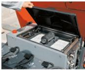
**Filter:** Easy-to-access electric R<sup>2</sup>S filter shaker system.
