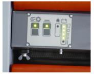
**Clearly structured:** The control display uses simple symbols to explain the different functions of the sweeper.
