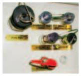
The lockable service center allows for easy service from ground level for: Fuel, hydraulic systems for hoist, steering and service brakes, coolant "IN" and engine oil.
