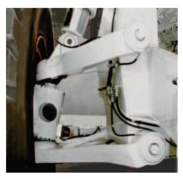
The T 252 features a "Double A-frame" Front Suspension. This unique geometry allows the tire contact point to move up and down in a straight line during travel and loading. Immediate and accurate payload weighing is possible since there are no side loads on the struts.
