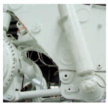
The unique Rear Wheel Suspension replaces the traditional nose cone with two Drag Links and a triangular Rear Control Arm. All forces from the rear axle are transferred into the truck frame in straight lines.
