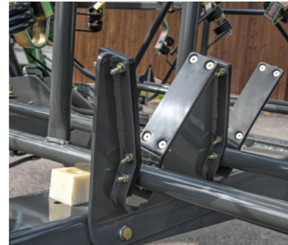
■ The Twister hoop guards, which are equipped with long-life bearings, fit perfectly into the special v-shaped brackets on the frame. (Only on Fendt Twister chassis version.)
