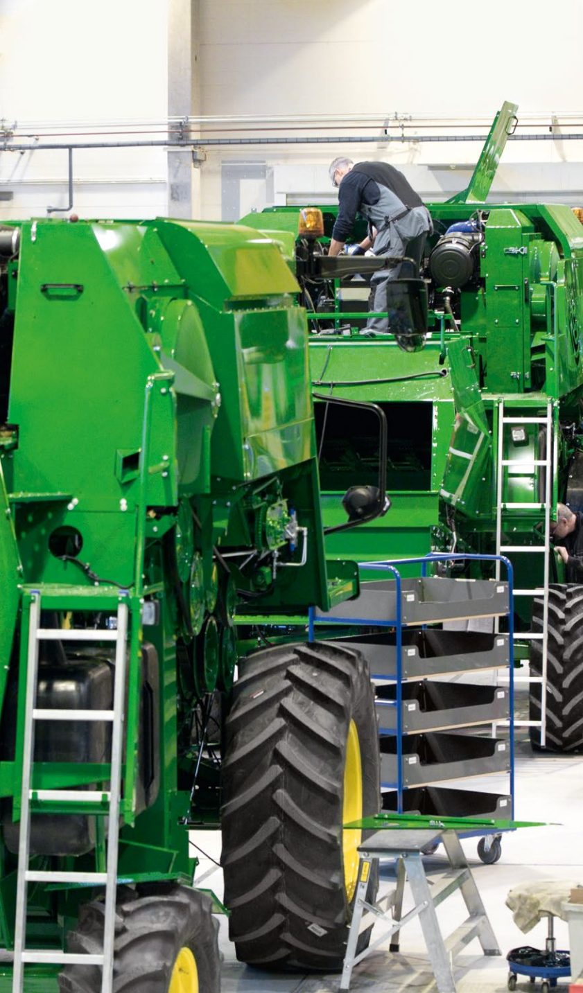
Every combine is custom-built for individual customers with plenty of options. The build card notes all the options and parts needed.
