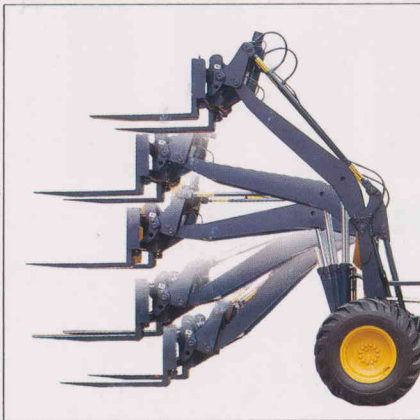
Parallel linkage keeps work equipment level.
